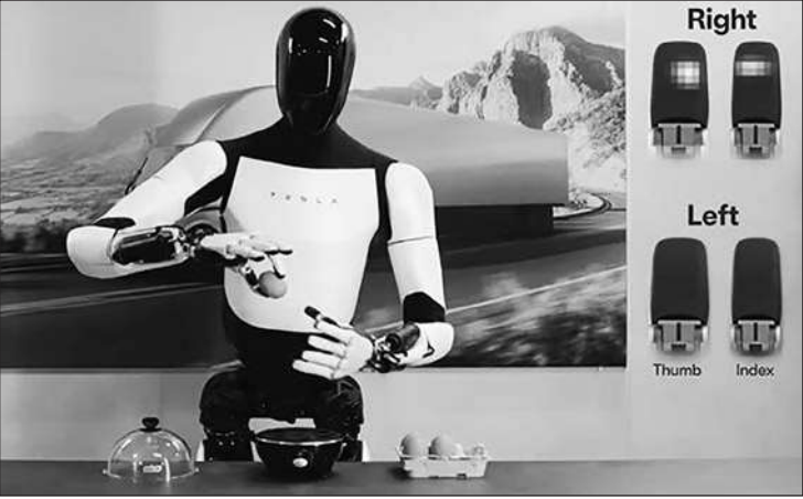
Optimus Gen 2 demonstrates sense of touch and dexterity. Photo Source: Tesla
