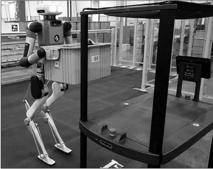
Digit is moving full totes from mobile robots to a conveyor at Spanx’s warehouse in Georgia. Credit: Agility Robotics
