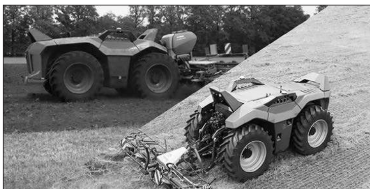
Krone and Lemken use Apex software to further develop the 'Combined Powers' project, autonomous drive vehicles and attachments that can take on various fieldwork. Credit: Apex
