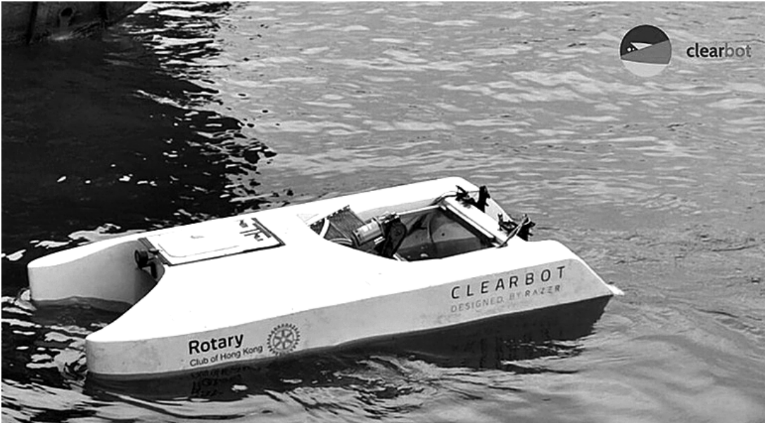
Clearbot Neo autonomously navigates the water and collects floating trash from its surface. Credit: Open Ocean Engineering
