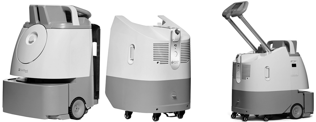
The Whiz Gambit autonomous mobile robot combines floor cleaning and disinfection capabilities into a single unit.
