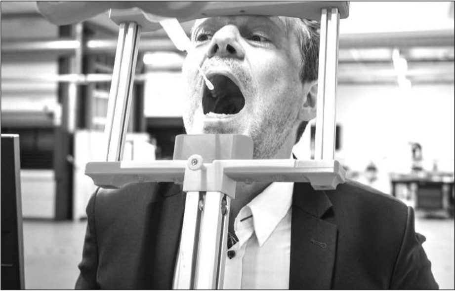
Lifeline Robotics’ throat swabbing robot collecting a sample from Co-founder Esben Østergaard. Photo credit: The Maersk Mc-Kinney Moller Institute at the University of Southern Denmark
