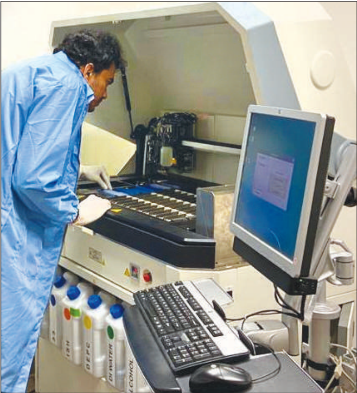
Testing quality of oligo probes used in COVID-19 test kits using Xmatrx infinity instrument manufactured by BioGenex.
