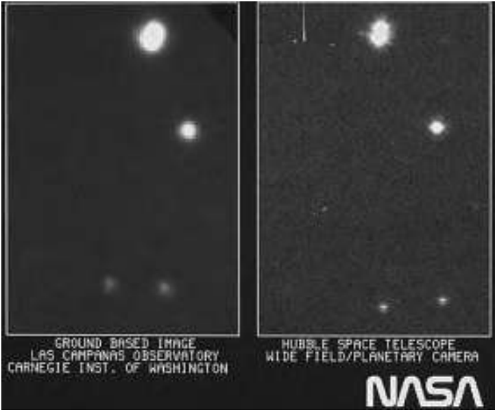
Hubble’s “first light” image. Even with the not-yet-corrected imperfections in its mirror, its images were generally sharper compared to photos taken by ground-based telescopes at the time. Image Credit: NASA
