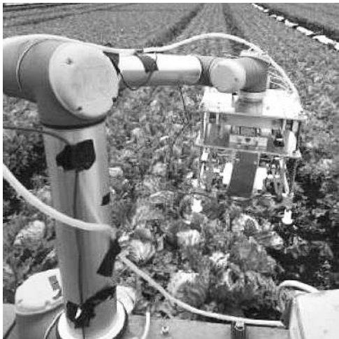
Vegebot uses machine vision to identify heads of iceberg lettuce. Credit: University of Cambridge
