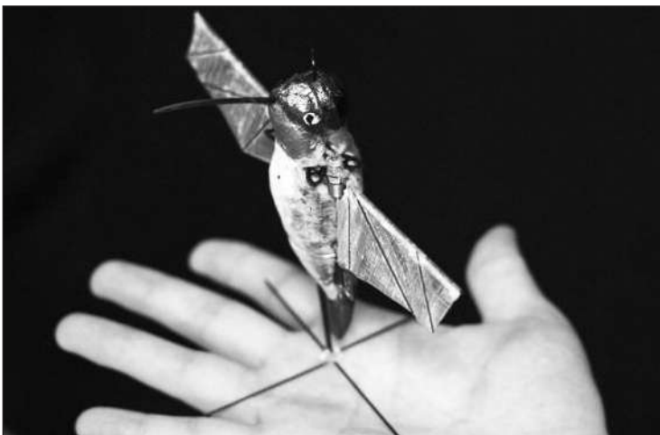
Purdue University researchers are building robotic hummingbirds that learn from computer simulations how to fly like a real hummingbird. The robot is encased in a decorative shell. Credit: Purdue University/Jared Pike.
