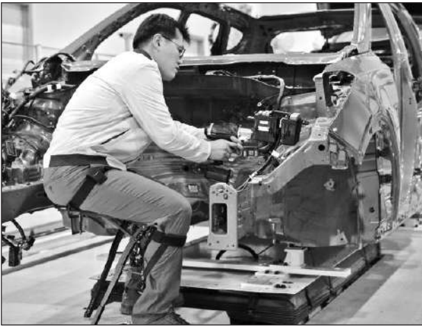
Hyundai is using the H-CEX industrial exoskeletons to relieve worker stress.
