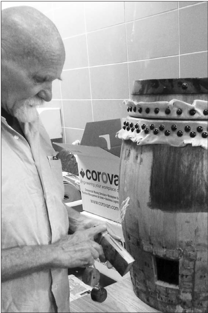
Terry Eustice with a demonstration drum, showing biscuit joinery
