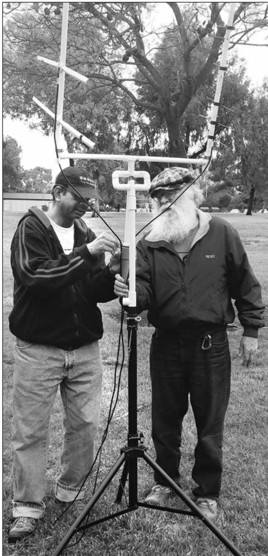
Umesh Ghodke (K6VUG) and Gene Arrillaga (KF6ZYD), both of Fremont, setup a homemade antenna for communications with satellites and the International Space Station (ISS).
