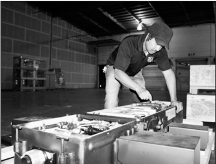
Train Control Electronic Technician Carlton Davis prepares a new switch machine prior to installation.
