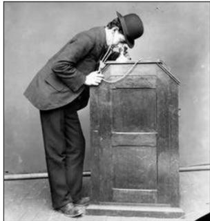
The 1895 version of the Kinetophone in use, showing earphones that lead to the cylinder phonograph with the cabinet
