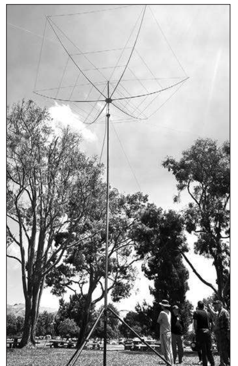
A group of enthusiasts and visitors marvel at the hexbeam before them
